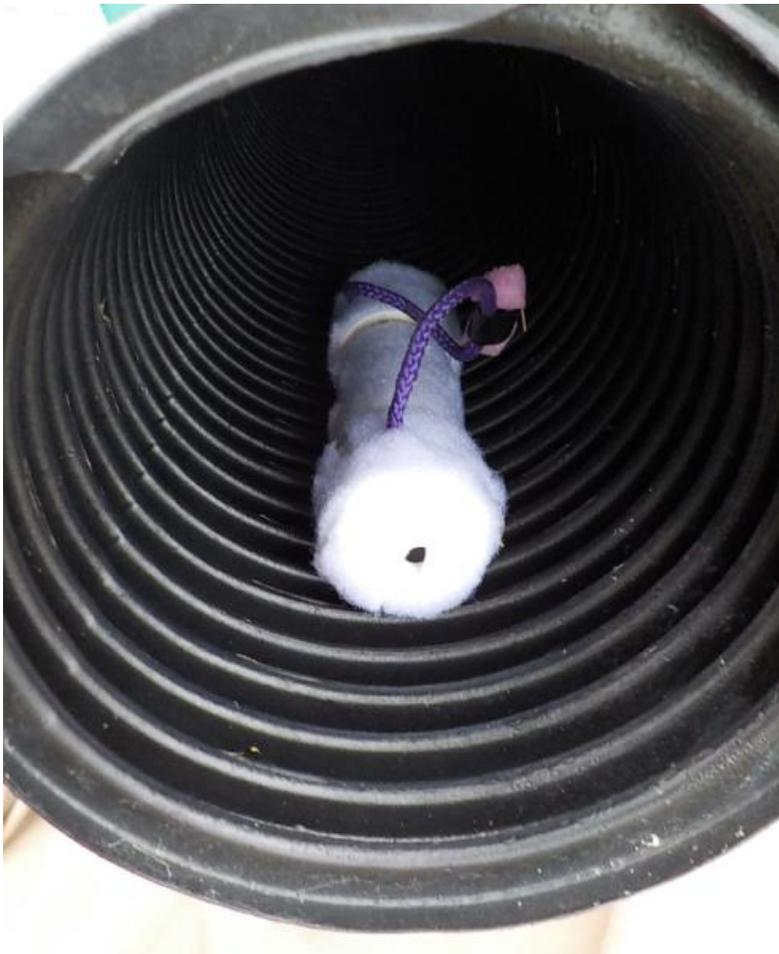
Sediment sample located at far end of drain pipe. Note: This photo is taken through the far end of the pipe (the covering on the far end has been removed).
