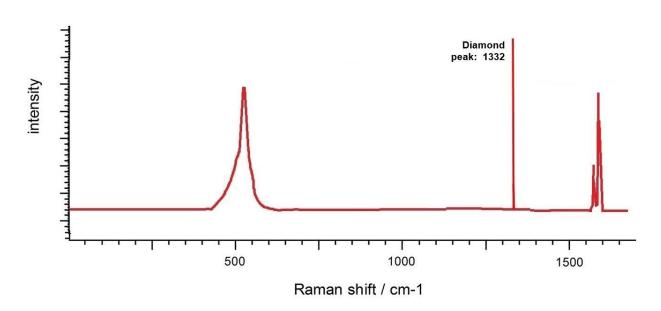
Raman spectrum of sediment contaminated with CdS (520-540 cm<sup>-1</sup>) and PCBs (1590 and 1575). Note the diamond peak (1332 cm<sup>-1</sup>).
