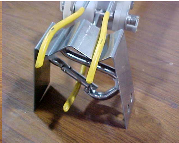
Figure 9b: Towfish Recovery Bracket in Gripper
