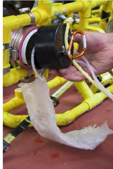
**Figure #11: Tow Fish Retrieval Device**
