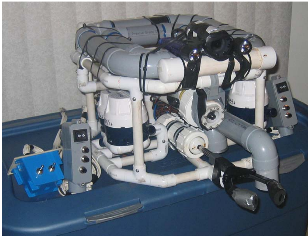
The ROV is flanked by the two Pilot controls and the blue box in the bottom left is the Co-Pilot control
