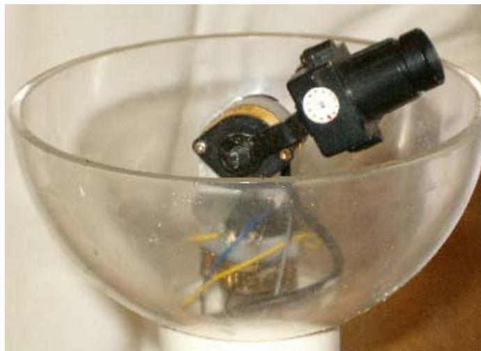
mounted to a small device held within a clear sphere. In this manner the pilot could monitor many different portions of the ROV as he traversed through tight spaces or around delicate items. Two P/T
