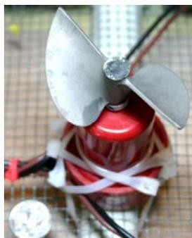
pitch. In water, one of these motors draws maximum amperage of 6.6 and sustained amperage of 6.0, producing a force of approximately 4.5 newtons per thruster. Because only one thruster will be employed for altitude, a 7.87 cm diameter propeller with 11.43 cm pitch is installed to maximize thrust. The amperage of this motor is currently unknown as it is a newly installed component on Proteus,
