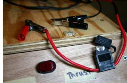
Throughout the duration of the project, there were numerous electrical anomalies that occurred. By using crimped quick connectors, we discovered it was extraordinarily easy to disassemble the electrical components and quickly seek out the source of the anomaly.
