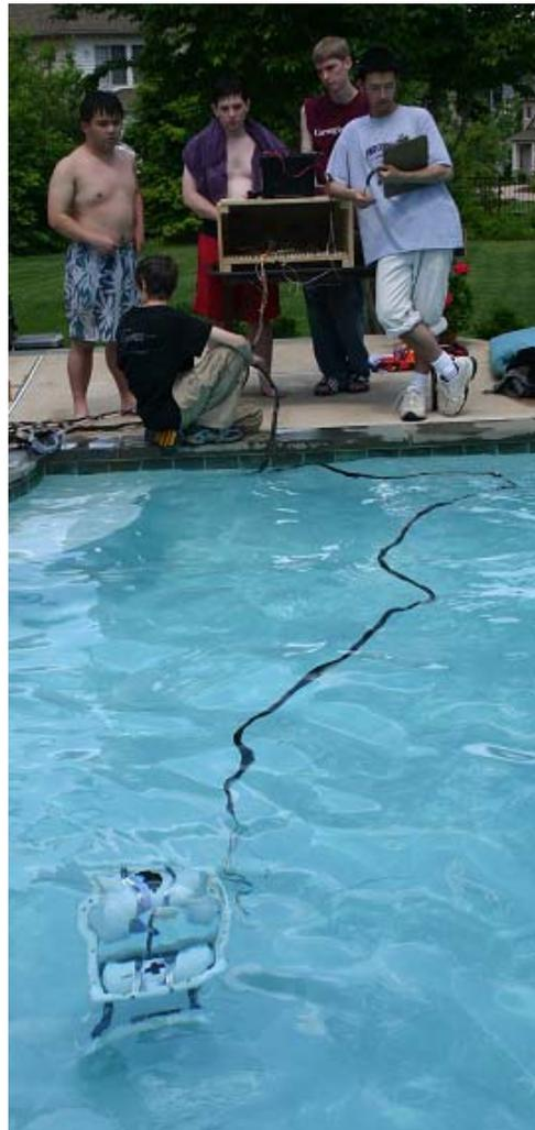
During our second major test of the Proteus, we encountered a decrease in thrust from each of our motors, which we attributed to the addition of the large PVC piping segments. We then decided to reevaluate our electrical schematics to
