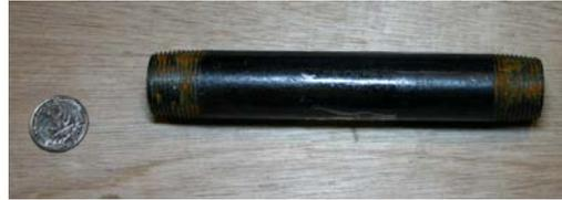
1.9 cm x 15.2 cm iron pipes are attached to the bottom of the craft, each weighing 225 grams (1.35 kilograms total). To counter the significantly negative buoyancy,
