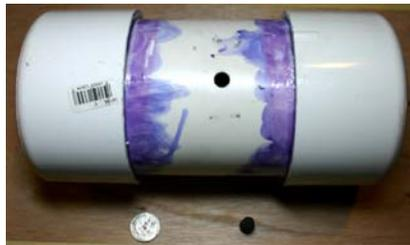
two segments of 10.16 cm diameter PVC pipes, each 28.00 cm in length with a mass of approximately 1.81 kilograms and volume of approximately 3.50 cubic meters, mounted perpendicular to the direction of thrust will serve as buoyancy compensators. Each tank has one 9.53 mm hole drilled to allow adjustment of the
