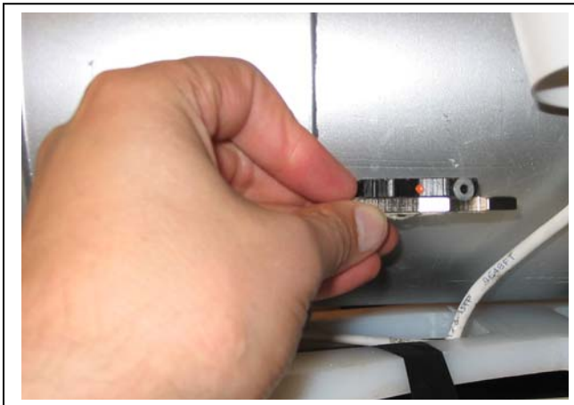
External magnetic switch to start the onboard computer after the termination can has been sealed.
