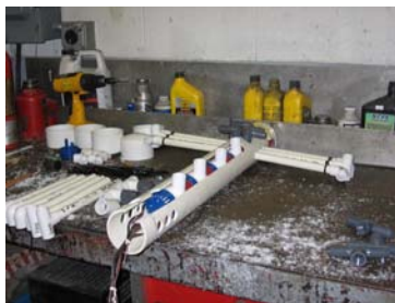
Fig. 2-2: Bilge pump system in construction.
