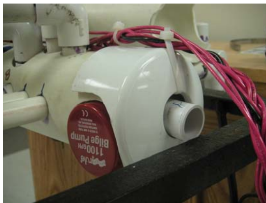
Fig. 5-2: Former reverse converted to forward thrust
