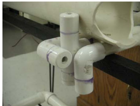
Fig. 5-1: Resistance caps on directional thrusters
