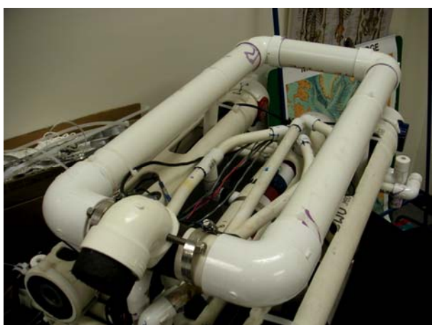
Fig. 5-4: Air/water-tight PCV ballast for added buoyancy.
