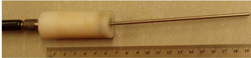
**Figure 5** RTD sensor package
