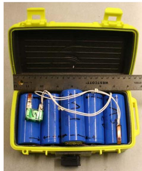
**Figure 3** Battery pack, complete with fuse
