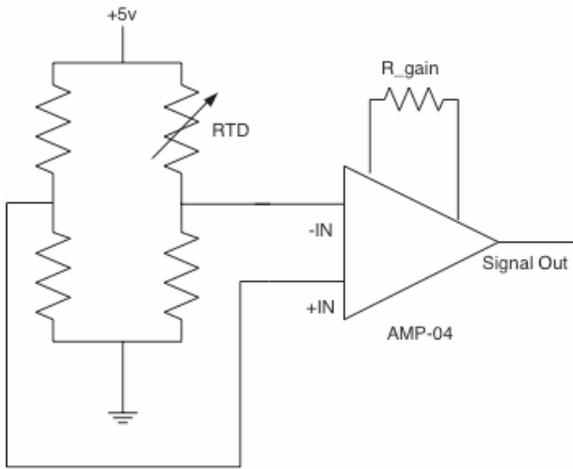
**Figure 6** RTD in Wheatstone bridge and amplifier circuit
