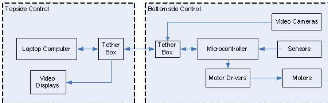
**Figure 9** Control System Layout
