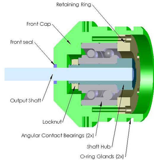
**Figure 11** Section view of Front Spindle
