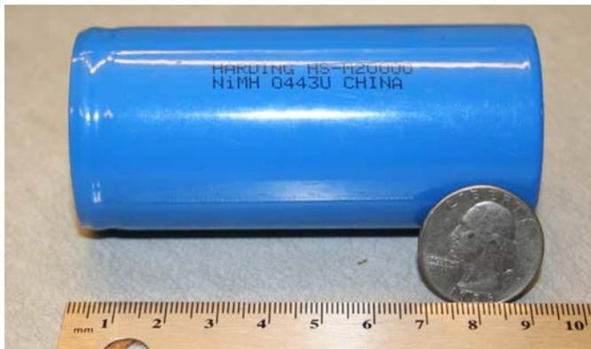
**Figure 2** NiMH 20 Amp-hour battery
