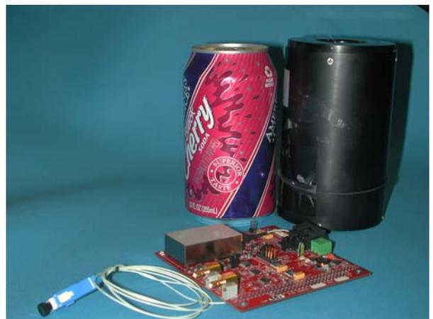
**Figure 8** Small fiber optic board and spooler
