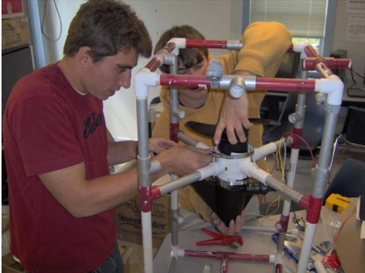
We chose the trolling motor because it has speed control. That way we are able to maneuver down the ice tunnel and reach the bottom very quickly, but not so fast that we will crash into the bottom of the pool. The Johnson motors are mounted transversely because it allows for small adjustments of our position. We can use them to strafe and to hover above a given point. We use the
