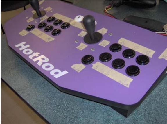
The method of “driving” the ROV that we will be using is through an arcade joy pad that plugs into the computer. This unit, called the HotRod, has two joysticks, and 18 buttons. It plugs into the keyboard port on the computer, and when something is pushed, it responds like a keyboard, by giving a character or something like Alt or Shift. This unit will be used mainly for the fact that it has so many buttons, so we can control more functions.
