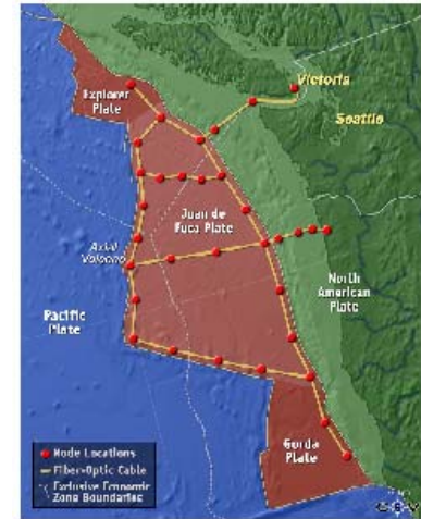
Figure 1. Bathymetric map showing the layout for NEPTUNE. The dots connected by lines denote the backbone cable and locations of the seafloor science nodes, respectively. The dashed line is the approximate location of the US and Canadian Exclusive Economic Zone.
