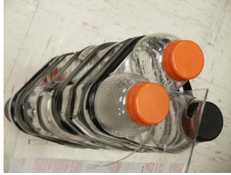
Fig.07– Gatorade ballast on right side of ROV frame
