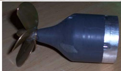
Water proofing the motors took very precise machining. As seen in the photo there is an oil seal and that was combined with an o-ring with just the right compression to stop leakage at the motor output shafts. With adjustments for weight and waterproofing our
