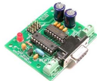
**Motor speed controller and servo controller used in ROV**
