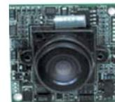
**CCD Camera used in ROV**
