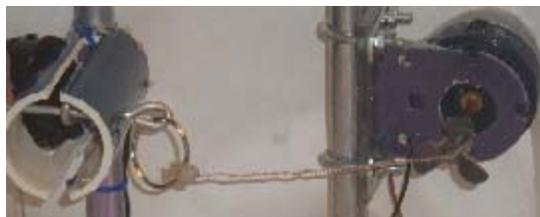
Figure 2: Pin pulling mechanism
