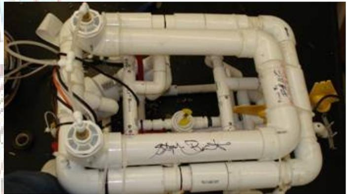
Top view. Notice the ballast tank (top u-shaped). It is tied down by zip-ties.
