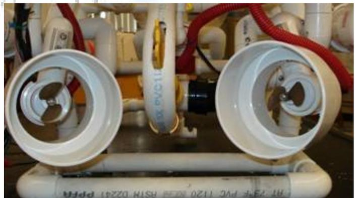
Angle mounted thrusters. Hard to see but are mounted inside the frame boundaries. Cowlings are also original. Might be disposed for weight issues.
