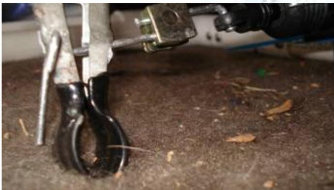
The newly made manipulator arm to grab instrument module box. Uses actuator from car doors.
