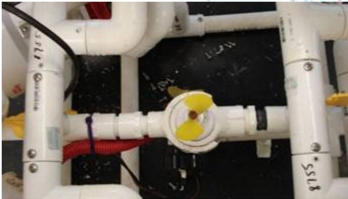
Top view. Notice the motor placement and the hand crafted mount. Motor is for up/down thrust.
