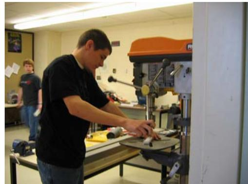
Drilling a hole into Lexan
