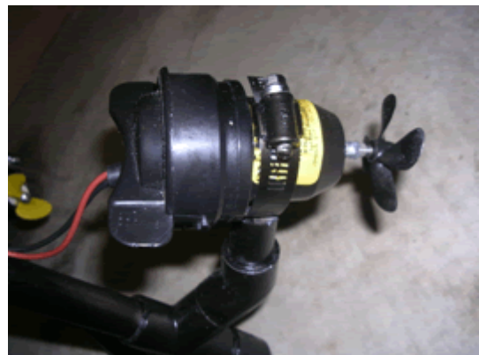
Figure 4: Modified Bilge Pump
