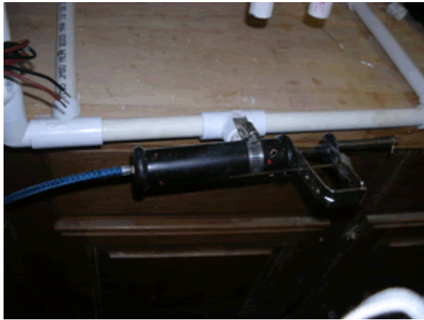
Figure 3: Pneumatic Actuator runs through the bar and just into the cylinder. It also runs through the pump handle. Just above the handle, on the guide rail, a spring was added. This spring acts to close the arm around an object when air is released. In order to open the arm, air is added to the cylinder, compressing the spring.
