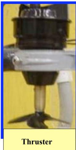
The team agreed on four Mayfair Marine 1250 GPH bilge pumps motors for our thrusters. These 12 V motors drew less than 1 amp out of water and about 5 amps underwater. We attached a four blade plastic propeller with a 70 mm diameter to each motor. Using a simple pull test, each motor was rated with a maximum thrust of 30 N. The motors are small and can be placed in the most efficient locations on the ROV.
