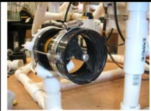
**Fig. 2-4:** Thruster with cort nozzles attached for speed and safety concerns, laterally placed motor for forward, reverse, and right and left movement
