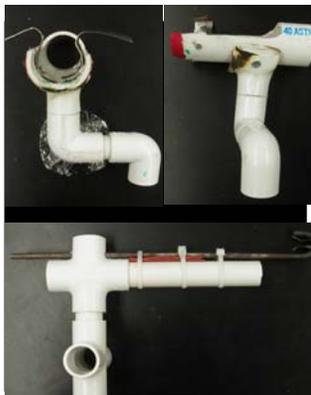
**Fig. 2-6:** Mission #1 arm, top two images of first appendage, this is used to pick up and insert tele-com connect, bottom image is of second appendage used to open door to the electronics module
