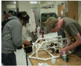
In building previous ROVs the team has discovered that polyvinyl chloride (PVC) pipes work best due to its rigid structure and durable strength. The team constructed the ROV frame from design sketches. After a proportional size reductions (Fig. 2-1) and seam sealing (Fig. 2-2) the frame ready for further construction.
