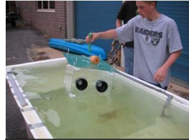
**Fig. 5-1:** Team member using spring scale to calculate the force (N) as well as weight (g) of the electronics module.
