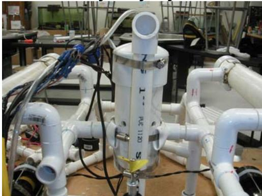
**Fig. 2-9:** Custom secondary buoyancy system modeled after a diving bell made specifically to compensate for weight of Mission # 1 electronics module.
