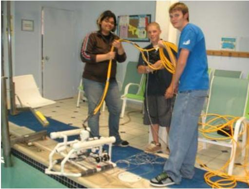
**Fig. 2-13:** Tether connected to the ROV via the central point of the bell system. Additionally PVC tube added to house the tether as it exits the vehicle, (see Fig. 2-9).
