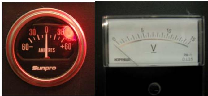
**Fig. 2-14:** Ammeter and volt meter on installed onto the control box of Aquafox in order to monitor power consumption while pool testing, and participating in the competition.
