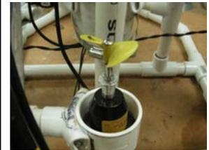
**Fig 2-5:** Central thruster used for vertical movement
