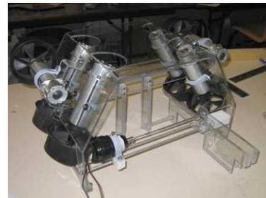
This design was used because the team decided to only use one multi-tasking tool to complete all tasks. This allows the ROV to be more compact and uses less materials and controls than having multiple tools. Polycarbonate was used for its durability and strength. The team decided to use proportional controllers to ensure that the tool works optimally and to reduce the amount of error.
