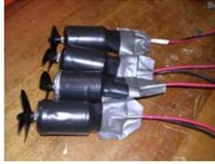
*Sealed, Heat Shrink Tubing Johnson Motors, April, 2006*
