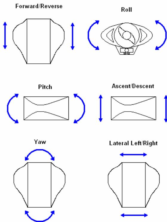
Because of the vehicle's ability to pitch and yaw, the pilot can also use the center thruster for linear movement in any direction. And because U D O is stabilized manually, the center thruster can be used for a quick ascent or descent by pitching vertically up or down and throttling forward the center thruster. This gives the pilot many possibilities for maneuvering.
