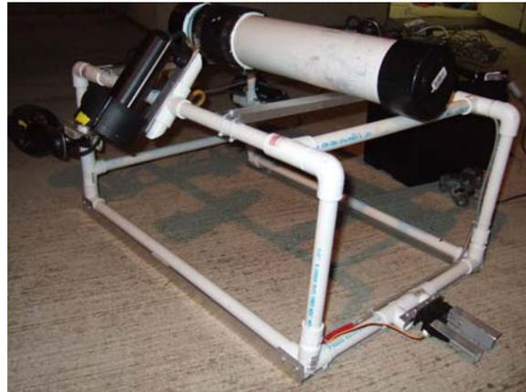
the horizontal bars for added structural strength and repositioned other horizontal bars for better equipment and thruster mounting options. Finally, we added "X" connectors to most of the places we thought we would want to mount thrusters to support both sides of the thruster and provide strong mounting platforms. To reinforced the thruster's mounts, we mounted the thrusters to angled aluminum, and then too the PVC frame.
