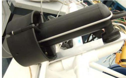
We also wanted thrusters that we could use repeatedly on later ROVs. We chose the Seabotix thrusters because they were designed to use an available amount of power to produce the necessary thrust for our mission.
