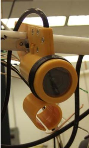
We are using a commercially available underwater camera. The camera is very similar to an X10 camera, but it comes manufactured with a built in lighting system and a waterproof housing using o-rings. Six white LEDs positioned around the camera lens comprise the manufactured lighting system. We modified the housing of the camera for mounting and, after examining the waterproofing, left it as it came.
