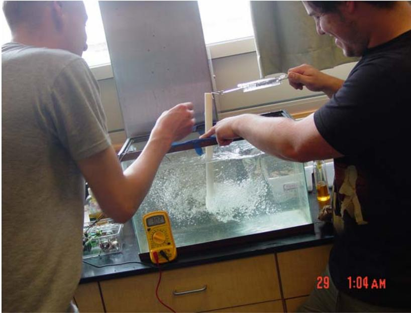
Figure 1.2: The motors being tested for thrust.
