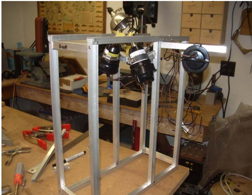
Figure 1.1: The two vertical motors are mounted at a twenty-three degree angle.
