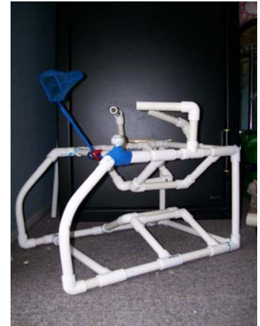
Figure 2. The frame of the ROV
