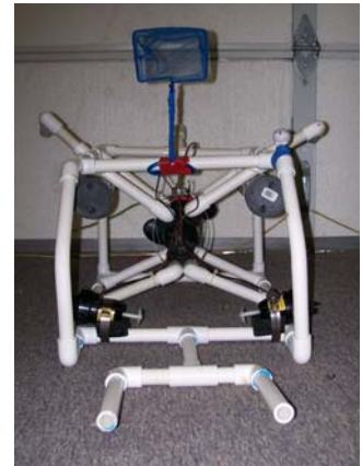
Figure 6. Thrusters added to frame
