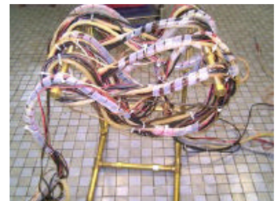
Tether management with nylon ribbon (flexible and reconstruct able)
