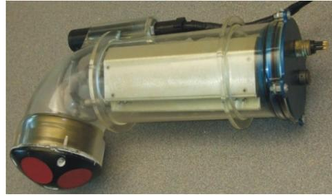
Figure 5 – DVL Hull
