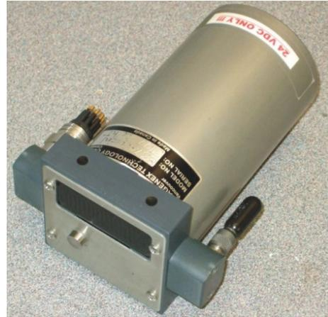
*Figure 9 – Multibeam Sonar*
