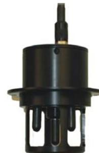
*Figure 11 – Passive Sonar*
