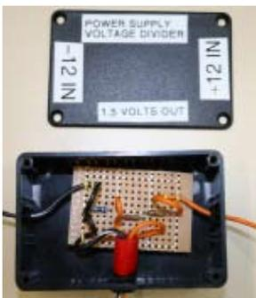
*power supply for temperature sensor*
