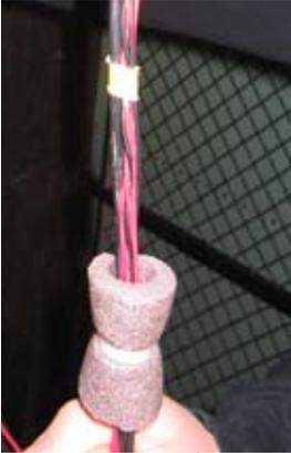
ROV tether and buoyancy foam
