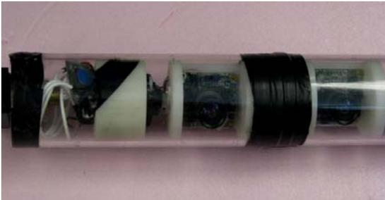
Figure 5. Stereovision camera system
