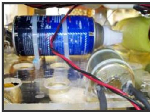
Figure 16: Solenoid and can of compressed air to fill container
