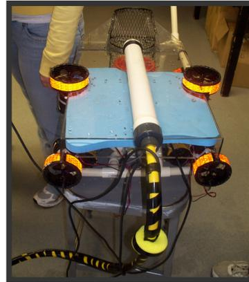
Figure 11: 2" PVC pipe where wires meet tether and exit the robot.
