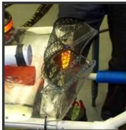
Figure 13: Lexan scoop with mesh basket
