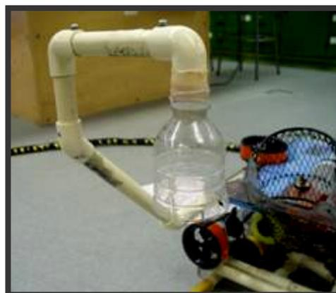
Figure 14: Arm that contains temperature probe
