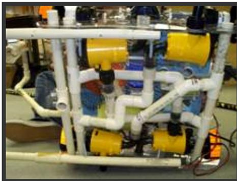
Figure 9: 500 GPH pumps that provide lateral movement
