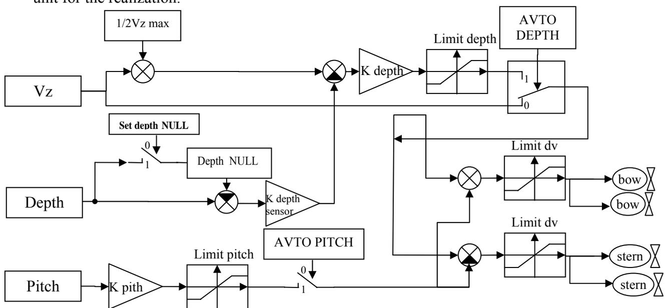
Fig. 16. Scheme of the vertical thrusters group control
