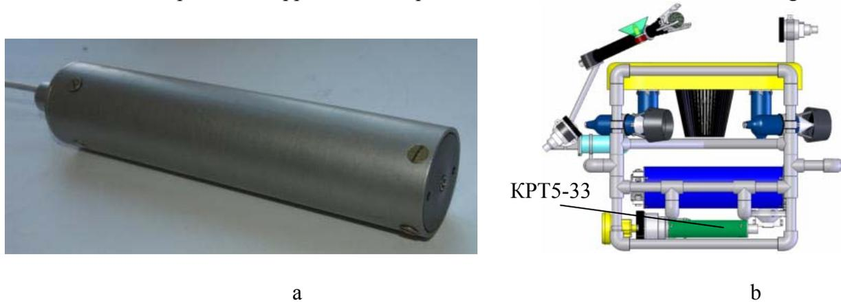
Fig. 8. The depth sensor: a) photograph; b) placement on the ROV
