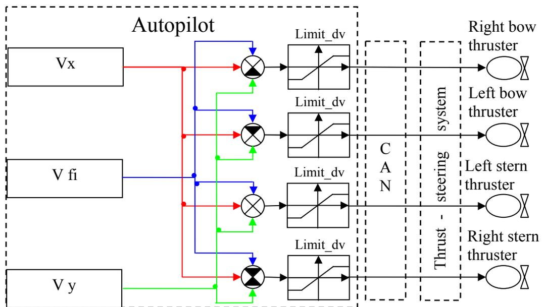
Fig. 18. Scheme of the horizontal thrusters group control
