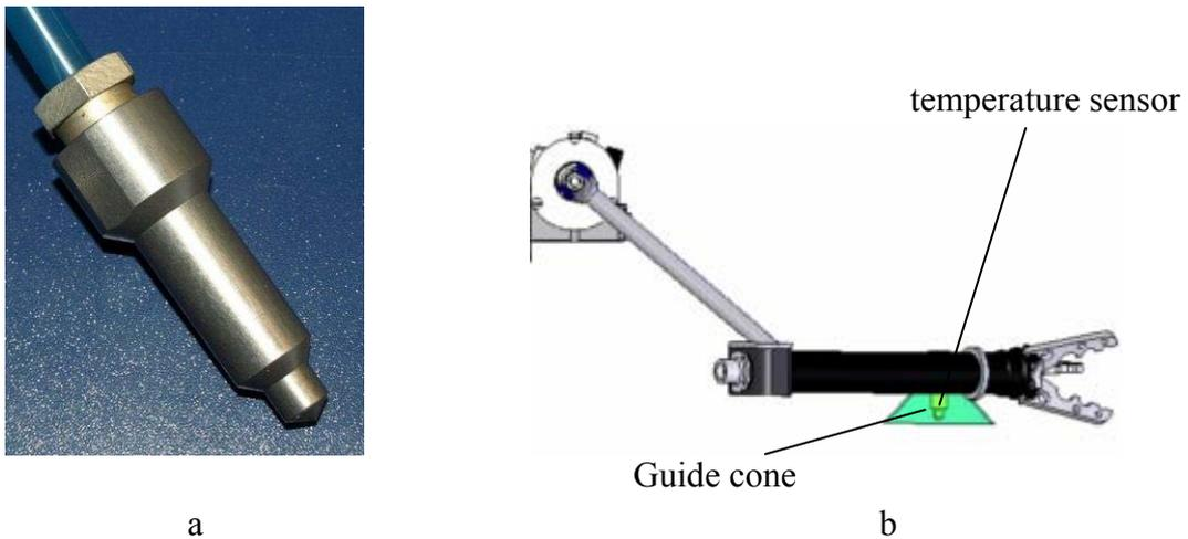
Fig. 9. The temperature sensor: a) photograph; b) placement on the manipulator
