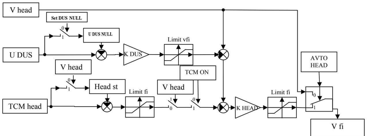
Fig. 17. Computation of the yaw control ( $V_{fi}$ )
