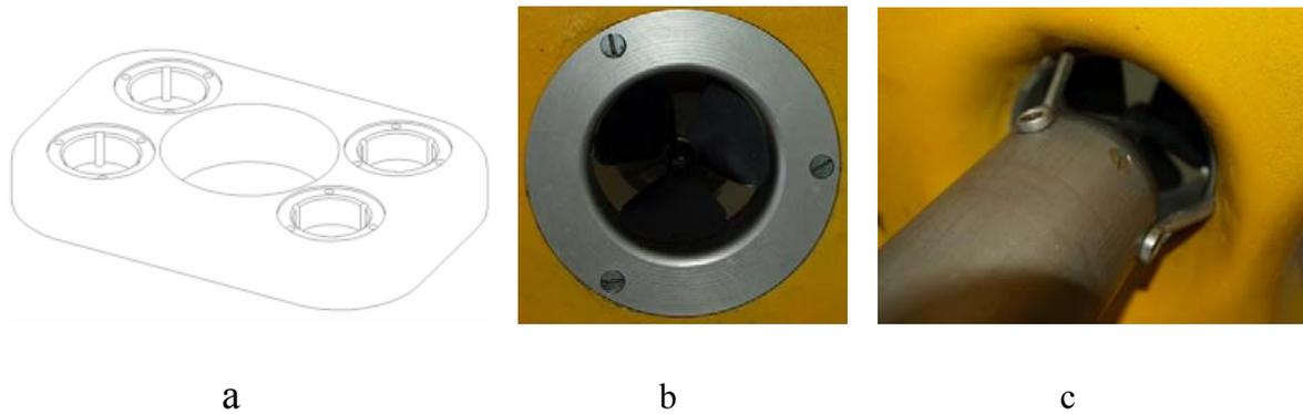
Fig. 7. Foam buoyancy: a) the model of buoyancy; b) water duct (plan view); c) attachment of the thruster to water duct
