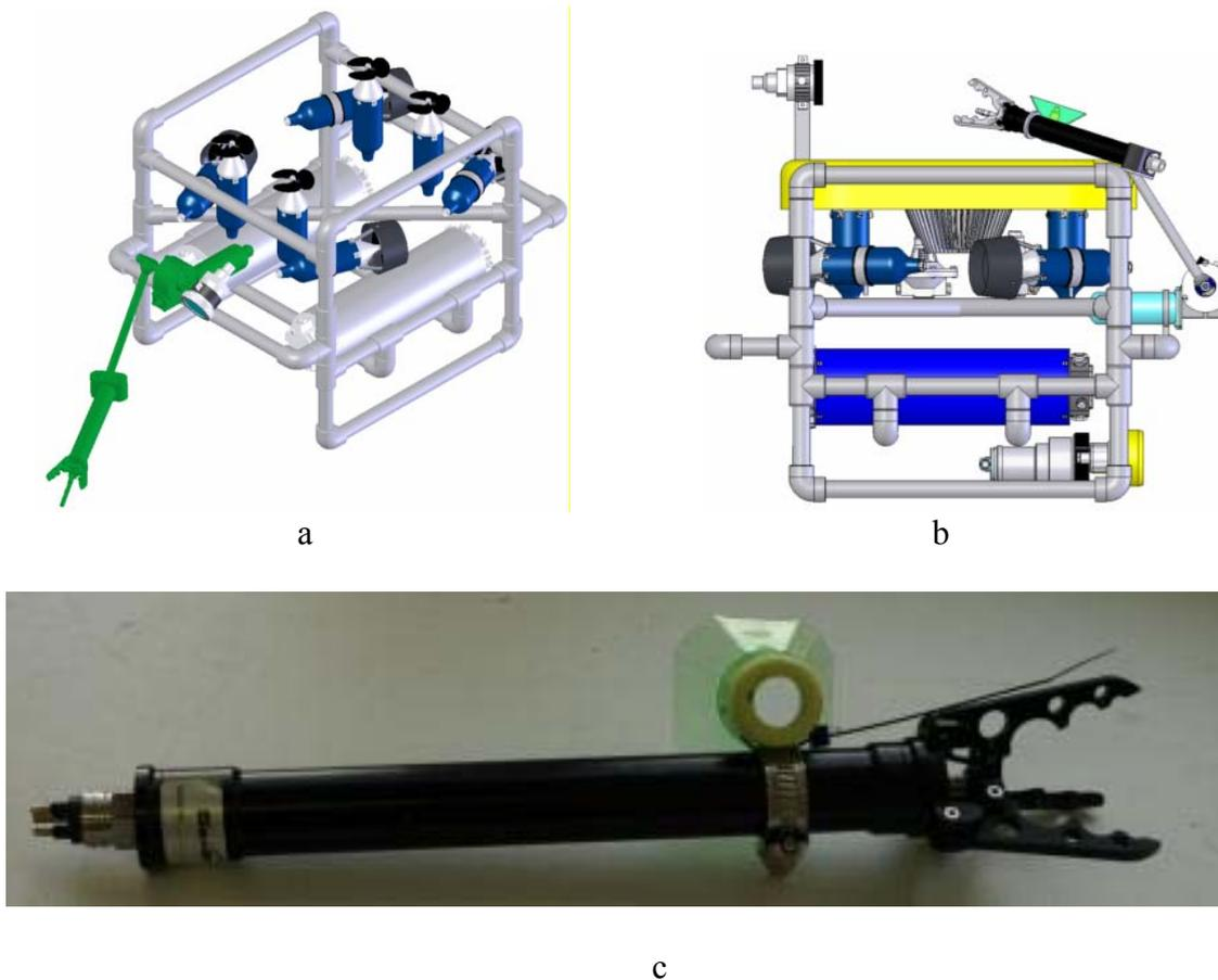
Fig. 4. Manipulator: a - position in common layout of the vehicle; b - transport position, position of samples reset into the basket; c – mechanical gripper
