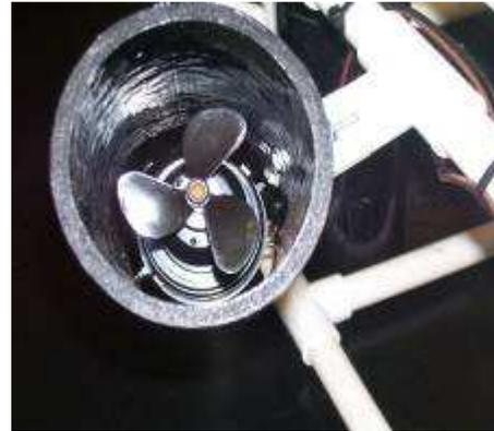
Thruster, propeller and safety housing
