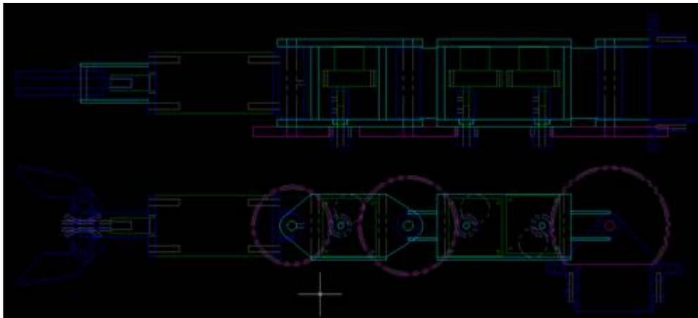
The arm portion of the ROV is constructed of aluminum, a plastic nylon, and stainless steel. The purpose of the arm is primarily collection of objects from the sea floor, with a secondary capability of taking a temperature reading from a temperature probe mounted on the arm. The arm consists of four axis's of motion and a gripping function. Each axis of motion is powered by a 12 volt DC gear motor with a 7189 to 1 gear reduction.
