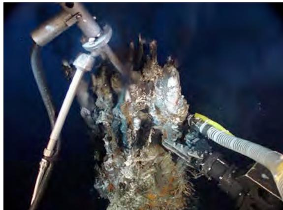
El Guapo hydrothermal vent on Axial Seamount. The vent water is being sampled and measured by ROV ROPOS.
