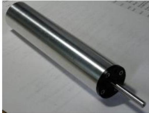
Fig 7: Partially assembled thruster, showing end cap
