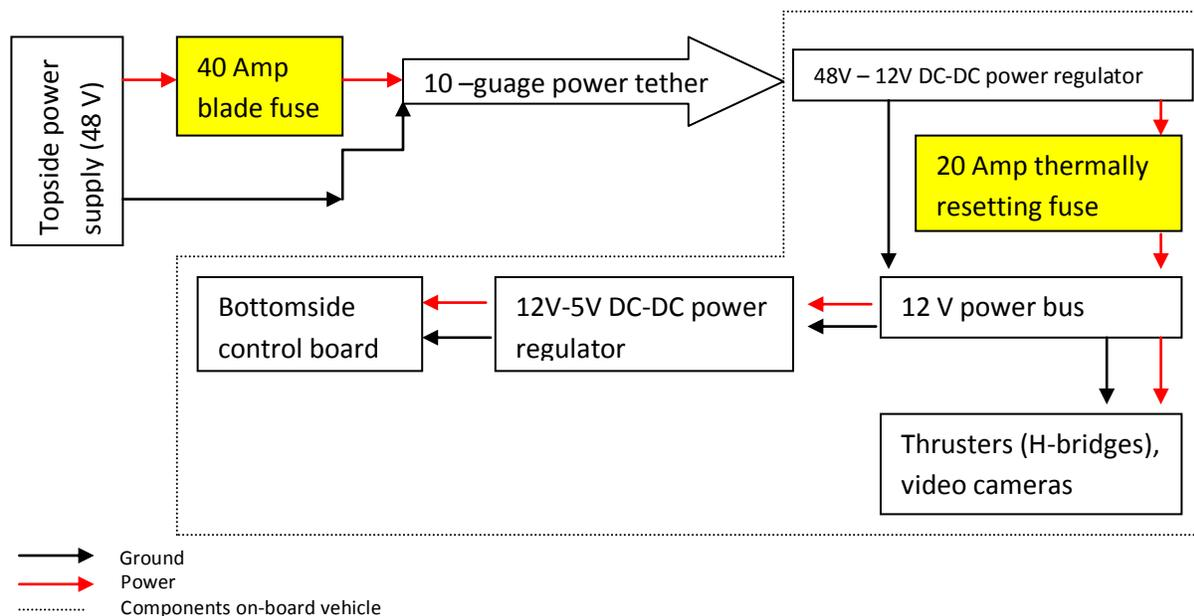
Fig 12: Electrical Schematic
