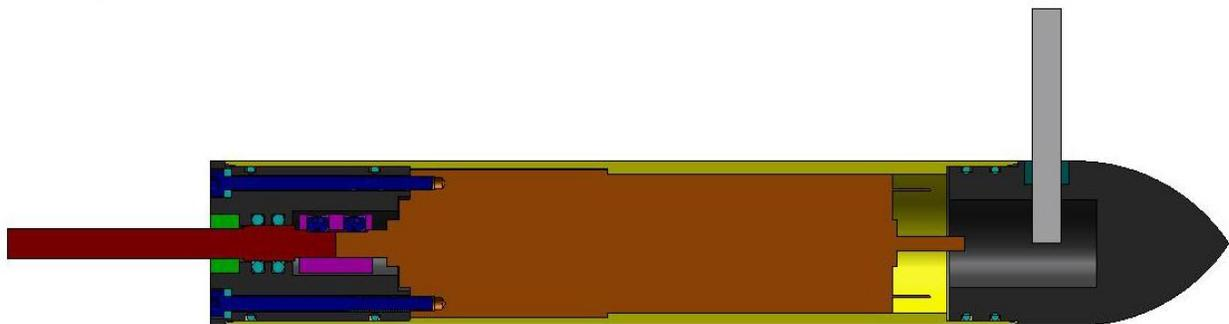
Fig 6: CAD model of thruster (section view)
