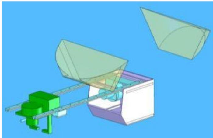
Fig 15: Gripper subsystems (Light blue- Linear Rail subsystem; Green- Grabber subsystem; Lavender- Variable Cargo Hold)
