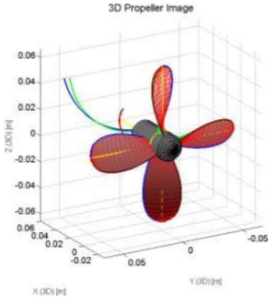
Fig 9: OpenProp geometry output
