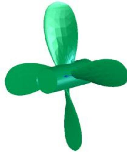
Fig 10: Final STL model of the propeller
