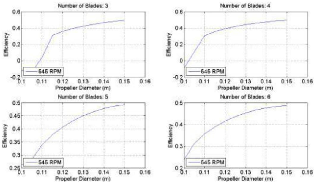
Fig 8: OpenProp parametric analysis output
