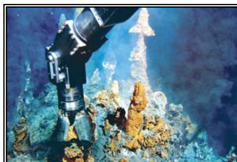
Victor 6000 collecting samples from the chimney of a hydrothermal vent ( www.gizmag.com ).
