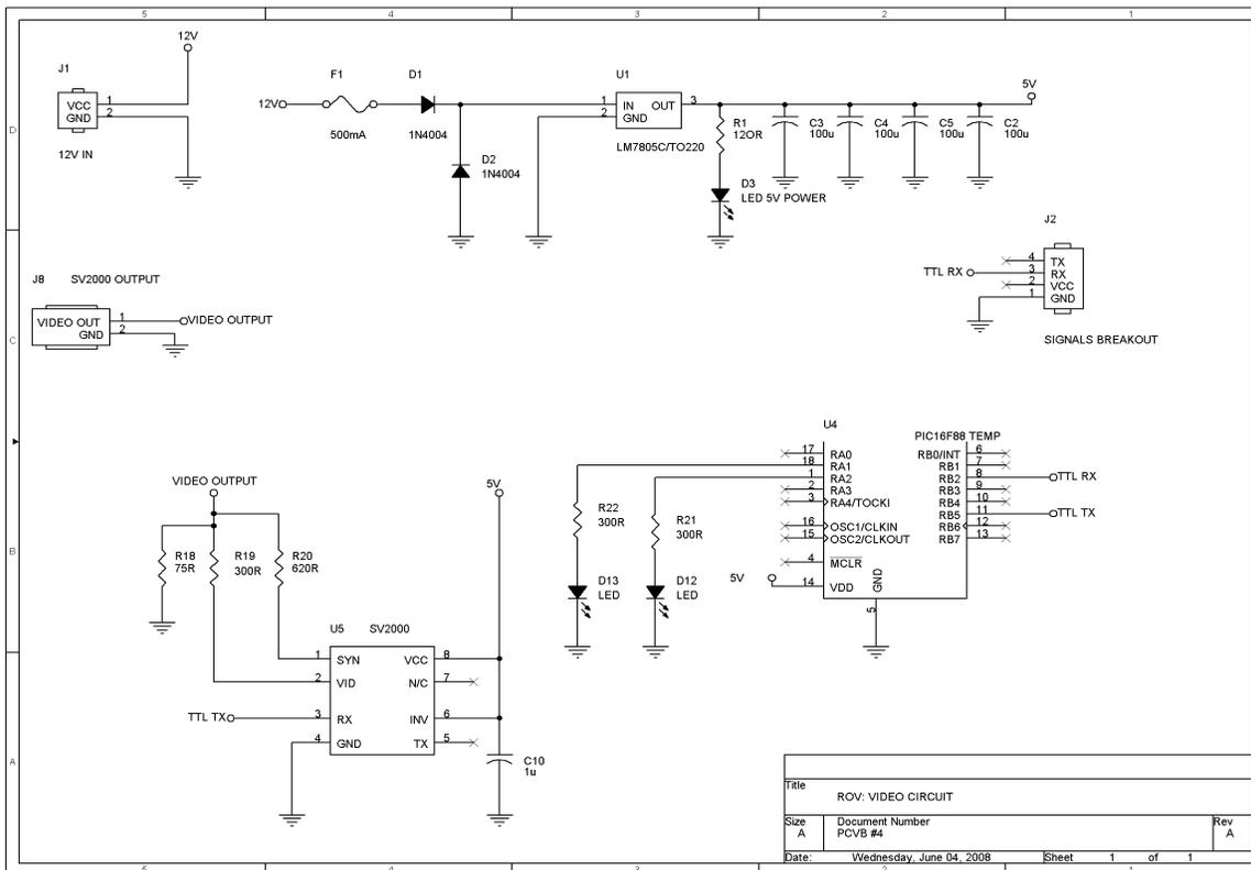
d. ROV video circuit schematic
