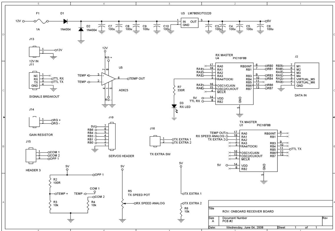
b. ROV onboard receiver schematic
