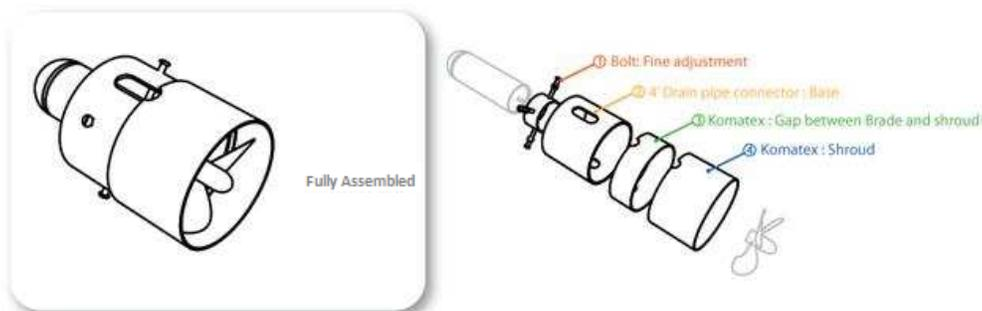
Fig 4 – Thruster shroud fully assembled and exploded view
