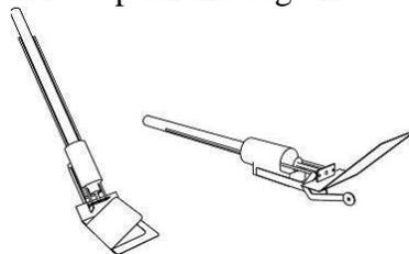
Fig 11 – Hamburger flipper manipulating arm
