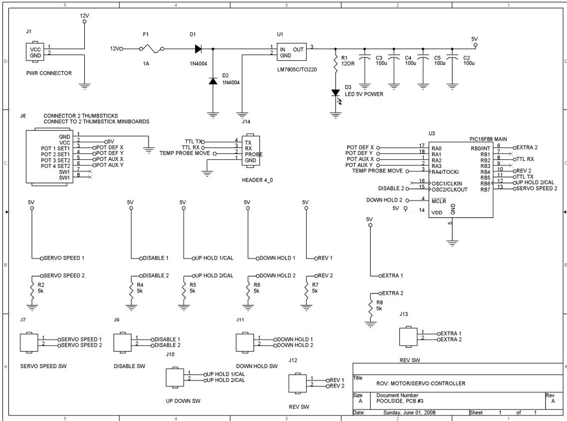
a. Motor/Servo Controller Schematic
