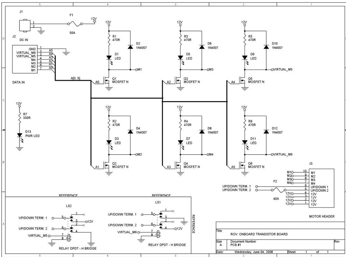
c. ROV onboard transistor board schematic
