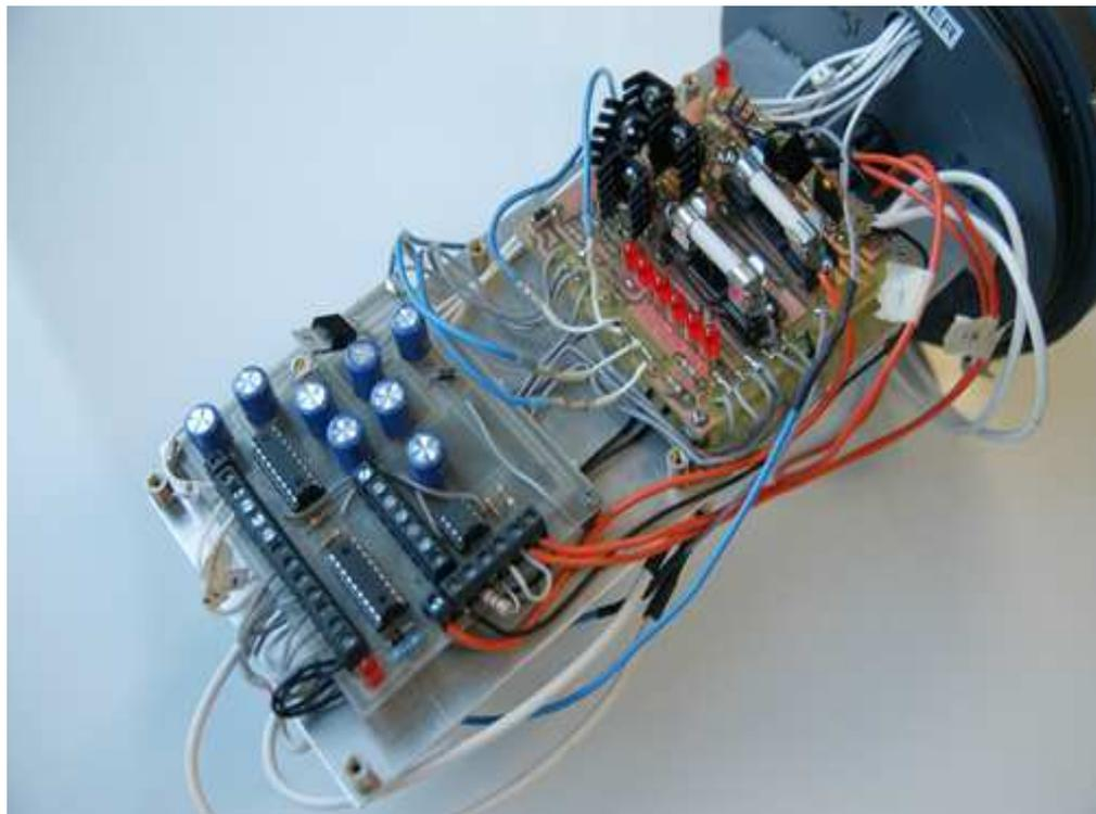
Fig 2 – ROV Onboard Electronics
