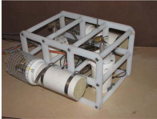
Figure 6 – Mounted Thrusters
