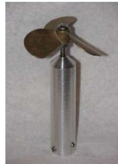
Figure 5 – Propeller on Adapter
