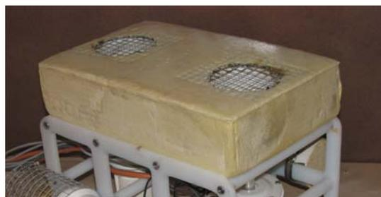
Figure 7 – Urethane Foam Positioned on ROV
