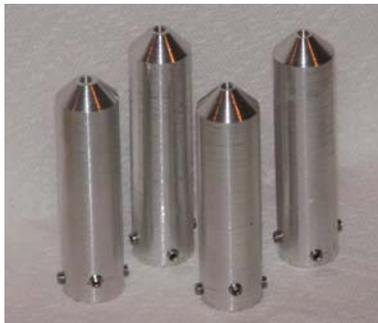
Figure 4 – Turned Aluminum Propeller Adapters
