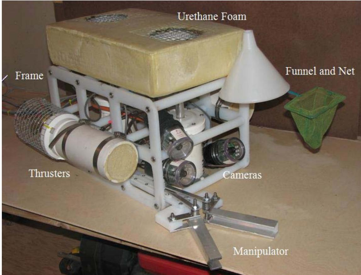
Figure 1 – Completed ROV with Labeled Components
