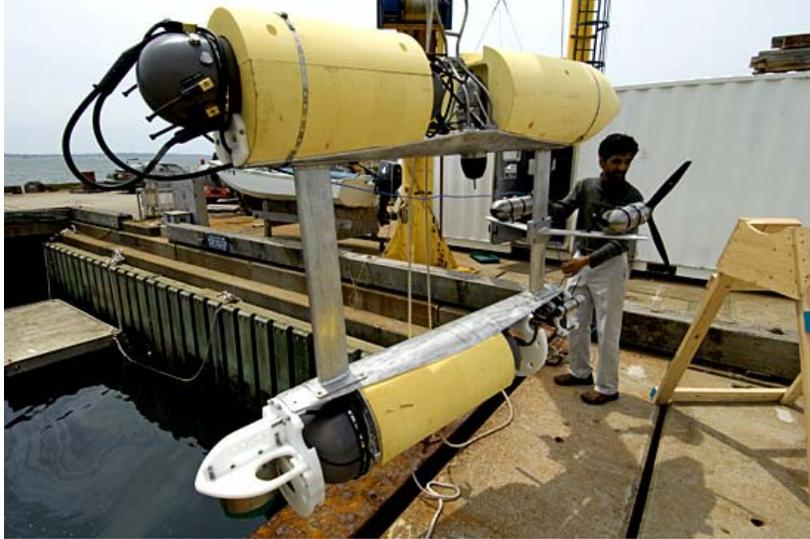
Fig. 5: The Jaguar during a dock test at WHOI<sup>6</sup>
