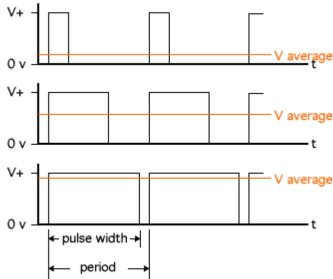
Figure 7 - PWM Waveform Example
