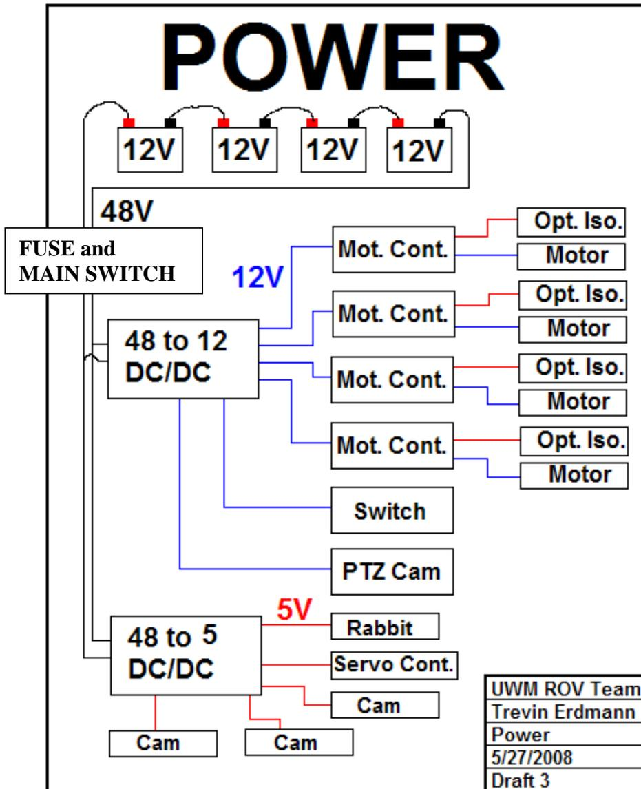
Figure 3 - ROV Power Distribution Schematic
