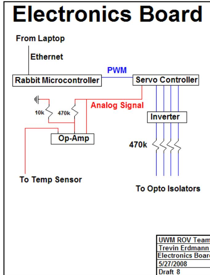
Figure 6 - Electronics Board Schematic
