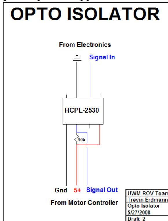
Figure 5 - Optoisolator Circuit Schematic
