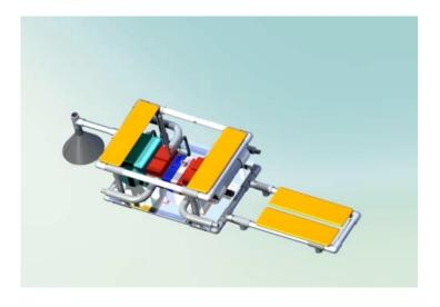
Isometric View of ROV Rendered in SolidWorks
