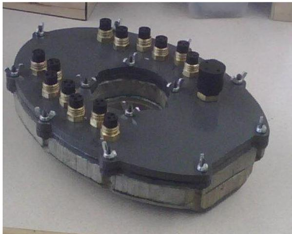
**Figure 4: The pressure hull bulkhead side**
