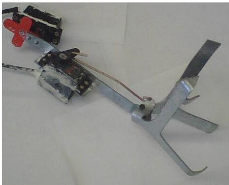
**Figure 7: A tool arm with servos and linkage**
