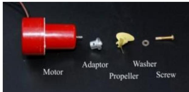
Fig. 2: Motor assembly
