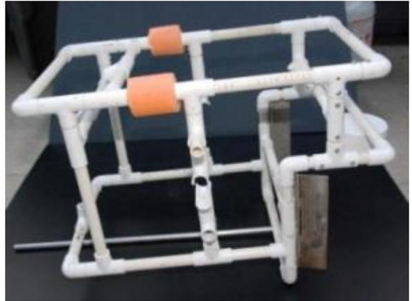
Fig. 1: Frame of the ROV
