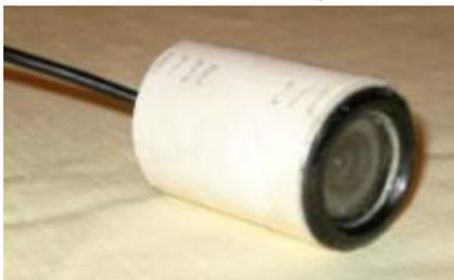
Fig. 4: A camera after waterproofing
