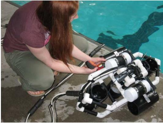
Figure 11 - Victoria Replaces Propeller
