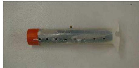
**Figure 10: Ballast tank**
