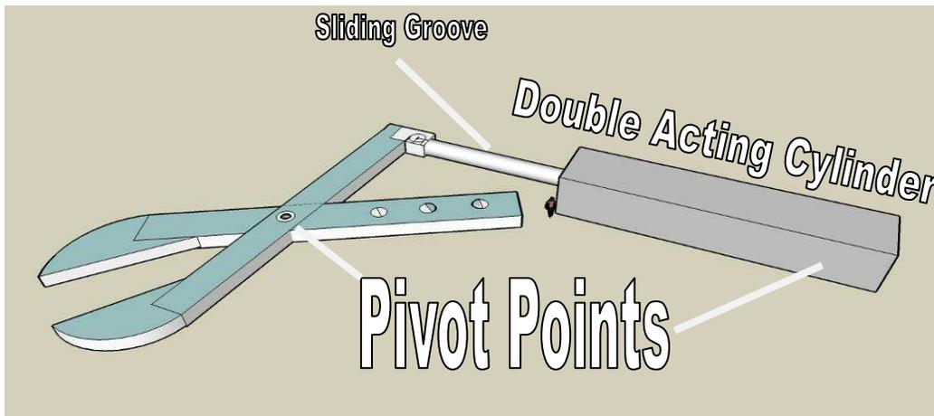
**Figure 7: Mechanical drawing of gripper**
