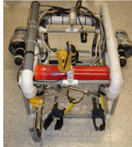
**Figure 2: Our finished ROV, top view**
