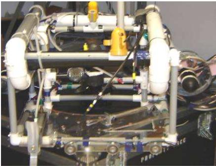
The biggest challenge we faced this year was the use of the electromagnets. Once we were familiar with the missions, our team brainstormed ideas to accomplish the tasks as efficiently as possible. We decided to try using three electromagnets to pick up the pods by the U-Bolts.
