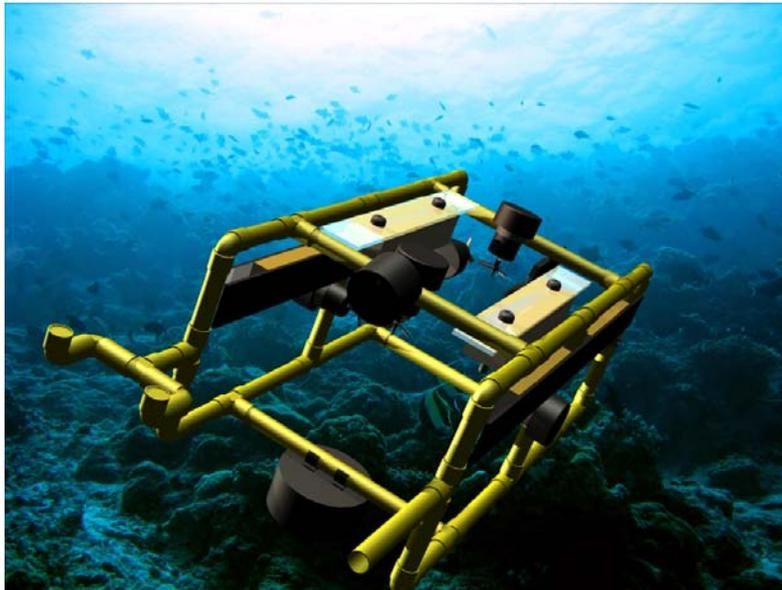
comes to rotating and opening the hatch. Indeed it is a piece of pipe protruding from the front of the frame we shall use to open the hatch and lift the weights out, effectively hooking them and carrying them out with it. The frame is made of 21mm diameter PVC tubing, as it is light, cheap and
