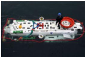
The LR5 Submersible Submarine Rescue Vehicle is an ROV employed by the Royal Navy and based near Glasgow. It has the capacity to carry up to 15 people to safety at an air pressure of 5 bar, and draws parallels to our ROV in that it is designed to take stranded crew from stranded submarines back to the surface, employing a mating skirt to do so – indeed in August 2005 it rescued 7 Russian crew members from the Priz submarine which had become entangled in fishing nets.
