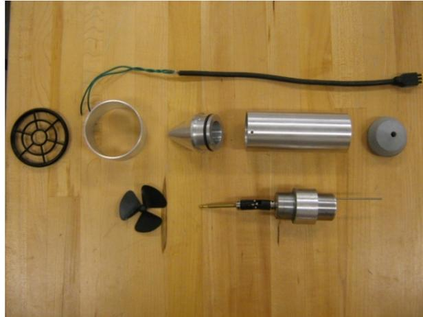
Figure 2: Thruster Components
