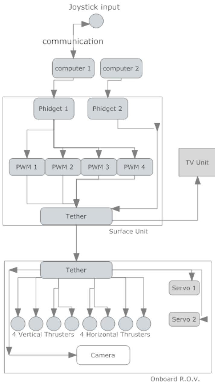
The propulsion of our ROV is controlled by one laptop computer running a Visual Basic program, which interfaces with a USB Joystick for control. The joystick movements are translated into code understood by our speed controllers, which distribute the correct thrust and direction to our R.O.V.
