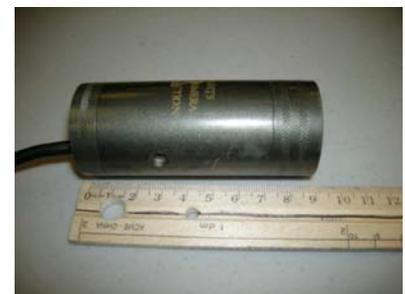
Figure 3: DSP Underwater Camera
