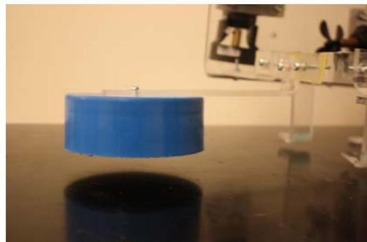
**Figure 13: Skirt used to “mate” with submarine in task 4**
