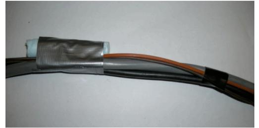
Figure 4: (Above) Old tether showing extra motor wire, buoyancy, temperature sensor, and camera wire. Figure 5: (Below) New Simpler Tether
