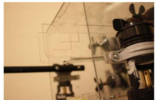
for easy insertion and retrieval. It is constructed from a single piece of Lexan bent into the desired shape. This enables it to remain lightweight and strong.
