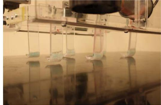
**Figure 11: (Above) Hooks Used to pick up ELSS pods for tasks 3. Figure 12: (Side Right) Hooks picking up ELSS pods.**
