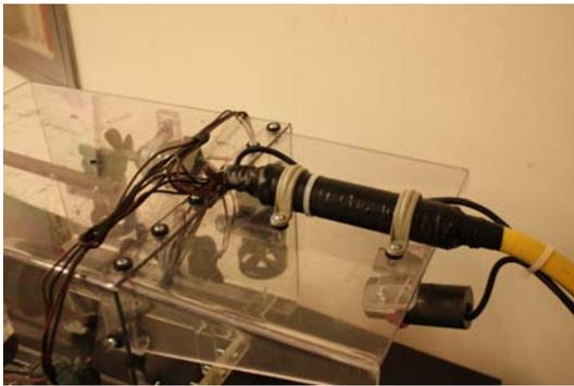
Figure 6: Waterproof tether connector
