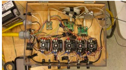
Figure 2: Phidgets and electronic speed controllers in the control box
